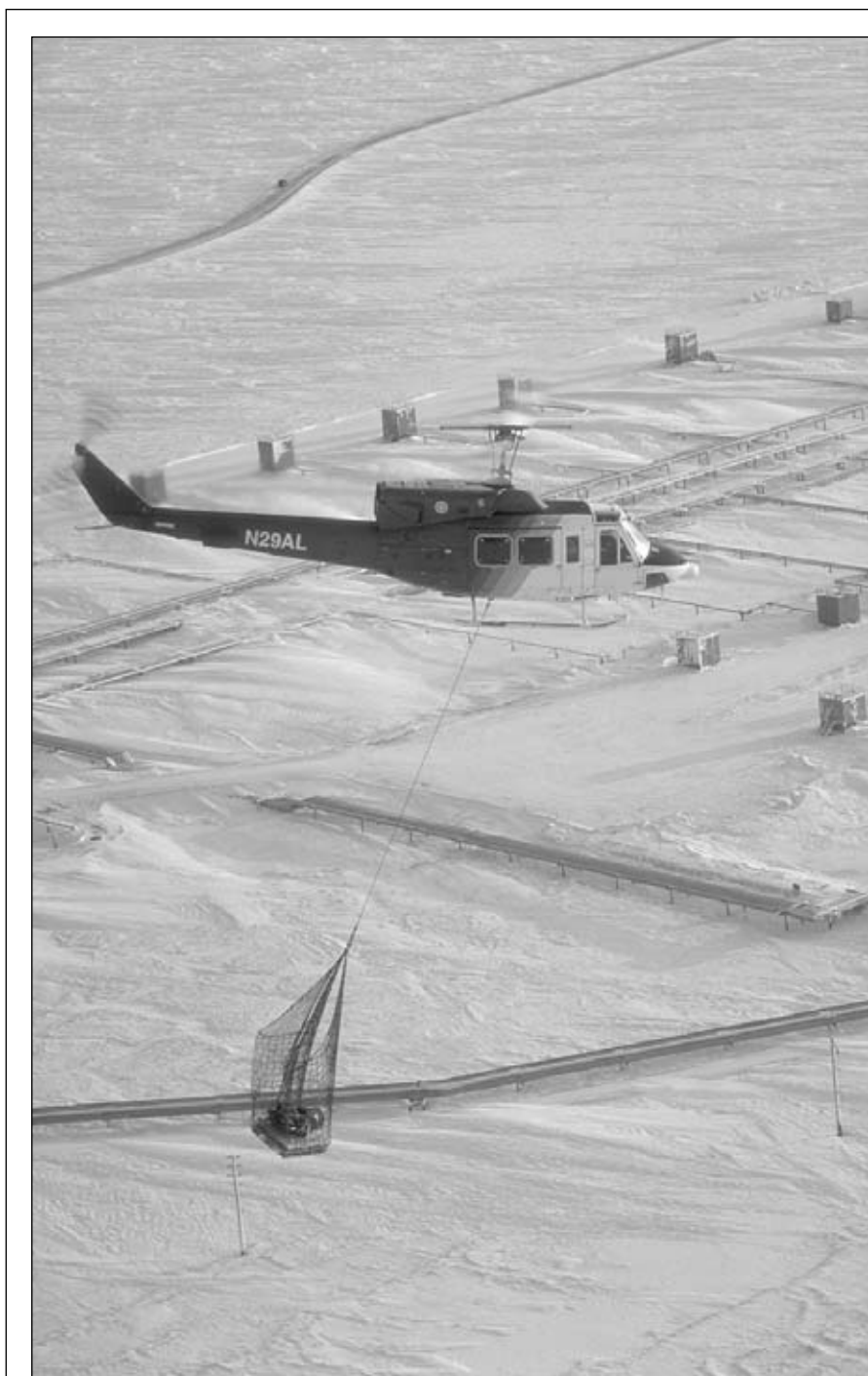
An Air Logistics Bell 212 carrying external cargo, North Slope Operations.
