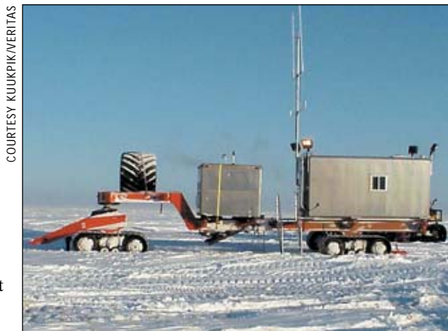
The recorder known as "the doghouse" is the administrative center for recording activity.
