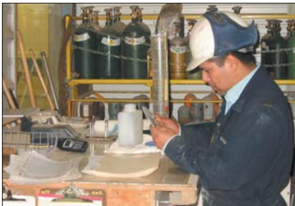
Ramp Fueler/ Yardman Roy Valerin testing jet fuel for prop-specific gravity before accepting a new load of fuel.
