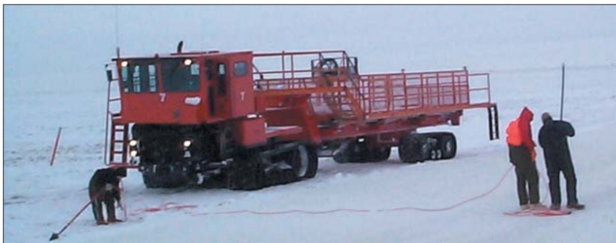
Challenger Tundra Tracker 195 rubber-tracked cable truck provides seismic cable support. The ground pressure exerted is 4.67 psi and cable capacity runs at 800 channels.
