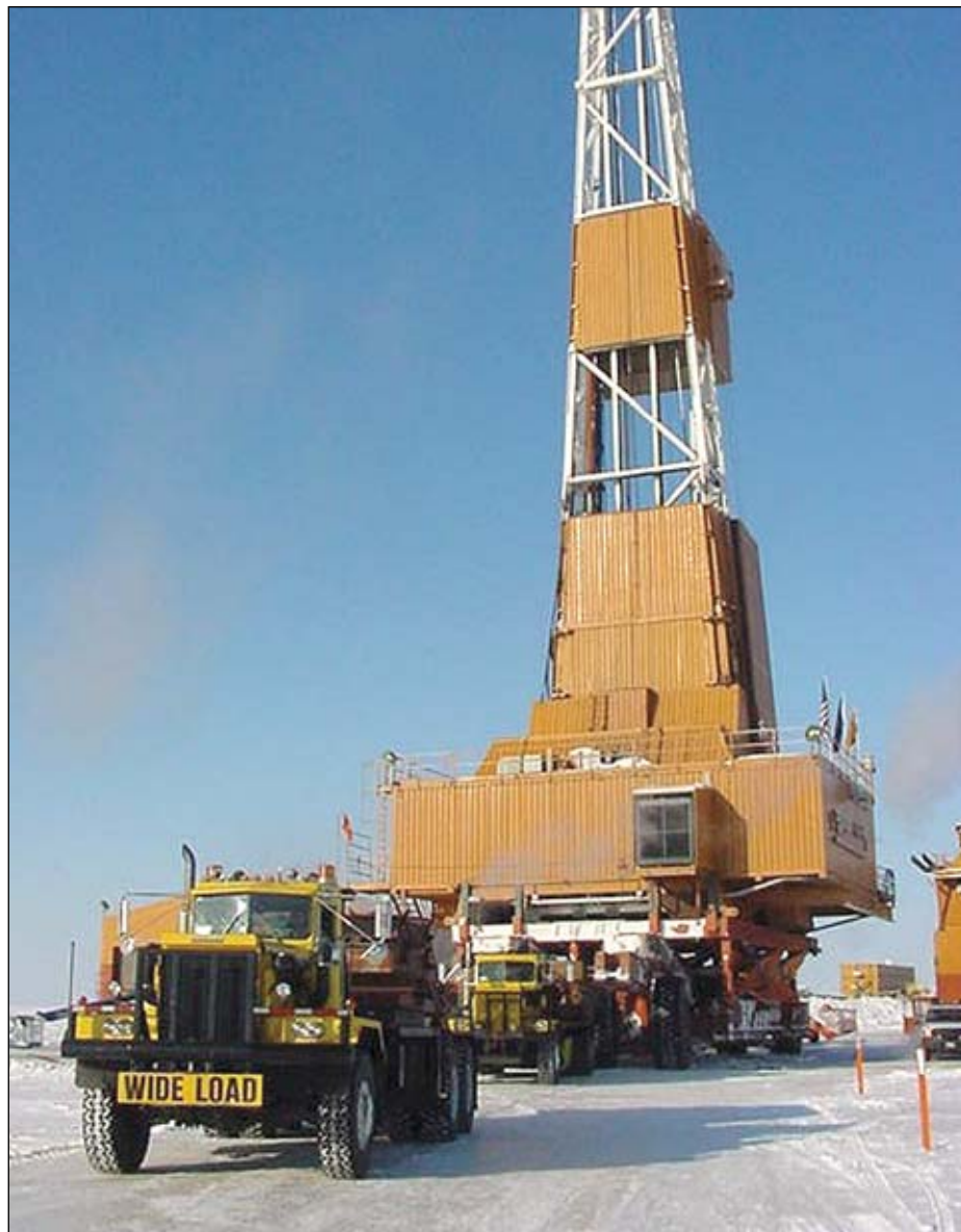
Doyon Drilling's Rig 19 rig floor transporter carrying the rig floor and drilling derrick.
