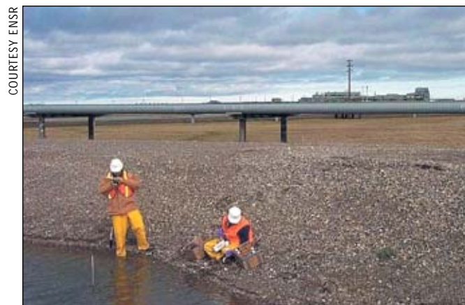
Surface water sampling in support of a reserve pit closure program on the North Slope
