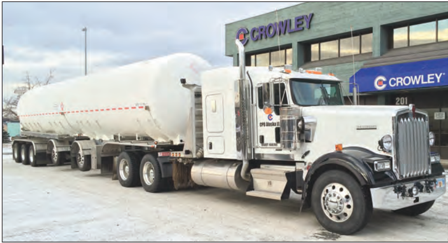
The prototype 13,000-gallon LNG trailer in Anchorage in December, ready for road trials in Alaska as part of the AIDEA Interior Energy Project.
