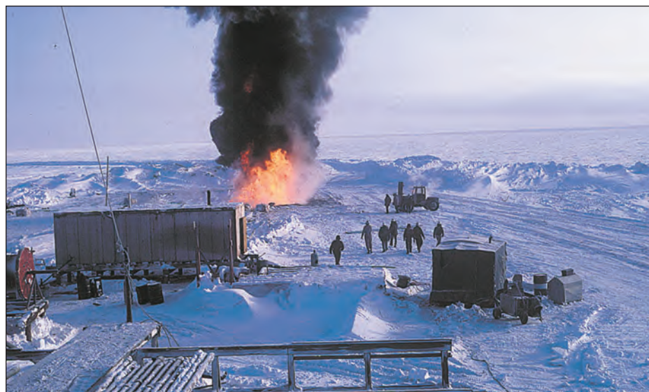
Drill stem test No. 5 on Feb. 18, 1968, recovered both gas and oil and clearly showed that oil could be produced from Prudhoe Bay State No. 1
