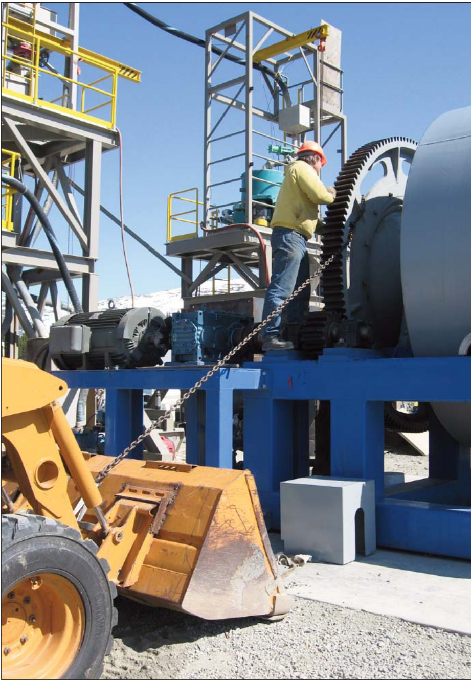
Workers align a SAG mill in May at the Yellowjacket Gold Project. JV partners Prize Mining Corp. and Eagle Plains Resources Ltd. reported completion of modifications to the project's 350-metric-ton-per-day mill facility. The partners expect to process 35,000 metric tons of gold ore at Yellowjacket in 2009.
