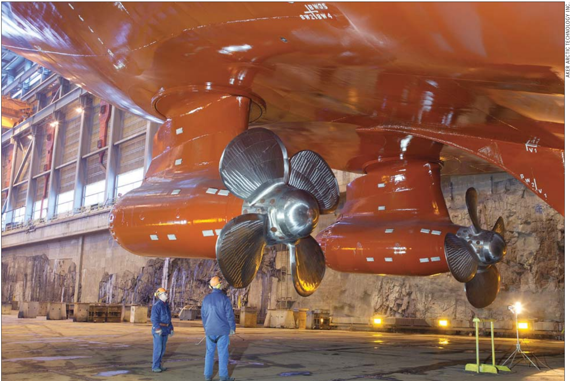
The azimuthal propulsion system on an icebreaker/supply ship. Twin diesel-electric "azipods" suspended under the stern can be swiveled in any direction.
