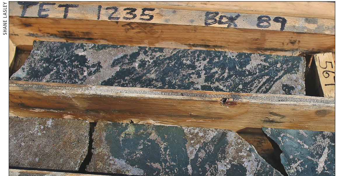
Core from a 17.3-meter section of a hole drilled into the Main Peak zone in 2012 that averaged 21.8 g/t gold, 7.4 g/t silver and 0.32 percent copper. This year, Peak Gold is seeking similar gold-rich skarn mineralization near the Main Peak deposit.
