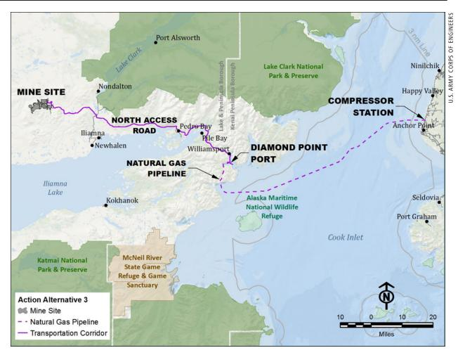
The subsea Cook Inlet portion of the Pebble Mine gas line would originate on the east side, making connection to existing gas pipeline infrastructure north of Anchor Point on the Kenai Peninsula. The subsea line would extend 75 miles to Ursus Cove on the west side.
