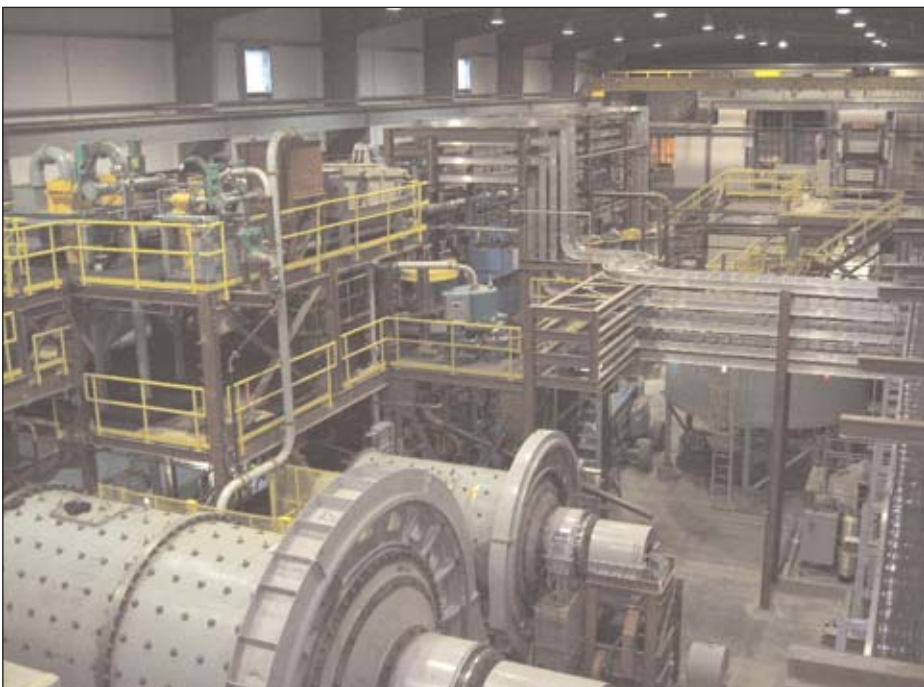
A look inside the new mill building at the Kensington Gold Mine. The primary and secondary ball mills are in the foreground.
