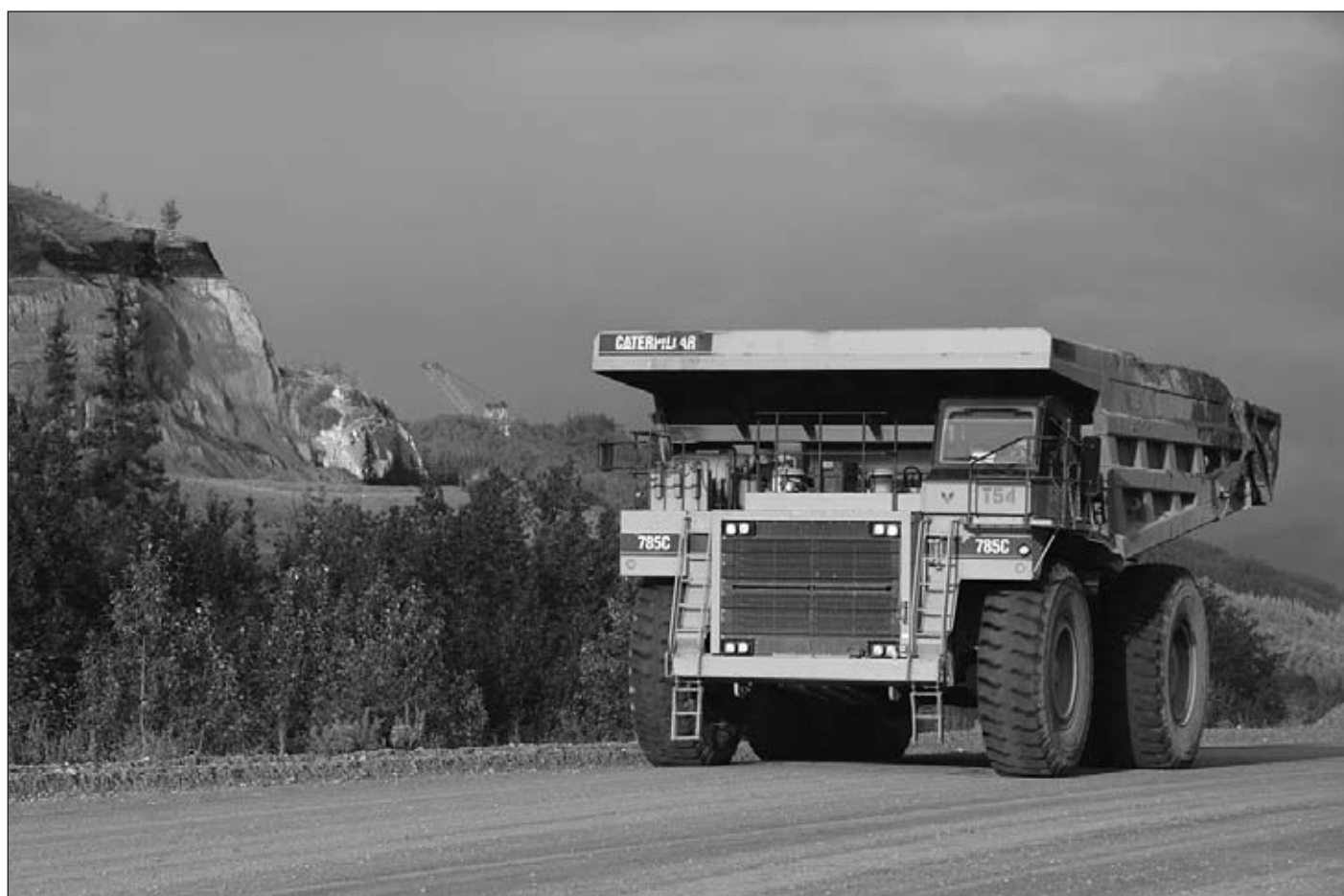
Installing tailgates on the haul trucks at Usibelli Coal Mine allowed larger loads of coal to be hauled for less fuel per load.
