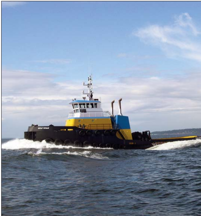
The most recent, fifth version, of the 120- foot, 5,000 horsepower Titan Alaska, is powered by a CAT 3516 engine.
