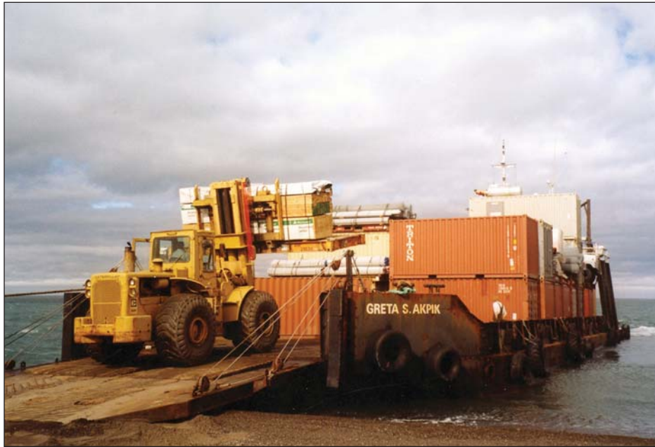
A forklift unloads cargo from the Greta Akpik, one of Bowhead's shallow landing crafts.
