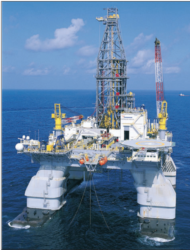
Transocean's Deepwater Horizon semi-submersible drilling rig, which drilled the Freedom discovery well in the Gulf of Mexico.
