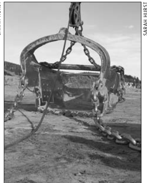
The bucket on the dragline is big enough to park a truck
