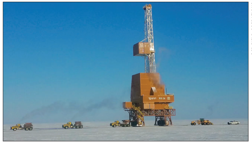
On March 27 the last piece of Doyon’s extended reach drilling rig, Doyon 26, left Deadhorse for the CD2 pad in the Colville River unit. The derrick and floor section module pictured here is being pulled by three large haul trucks cabled together.
