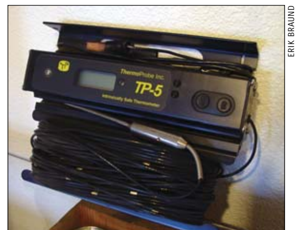
One of many updated products available at NEI Fluid Technology, the ThermoProbe TP-5, a digital thermometer used in determining temperatures in large fuel tanks and in custody transfer.
