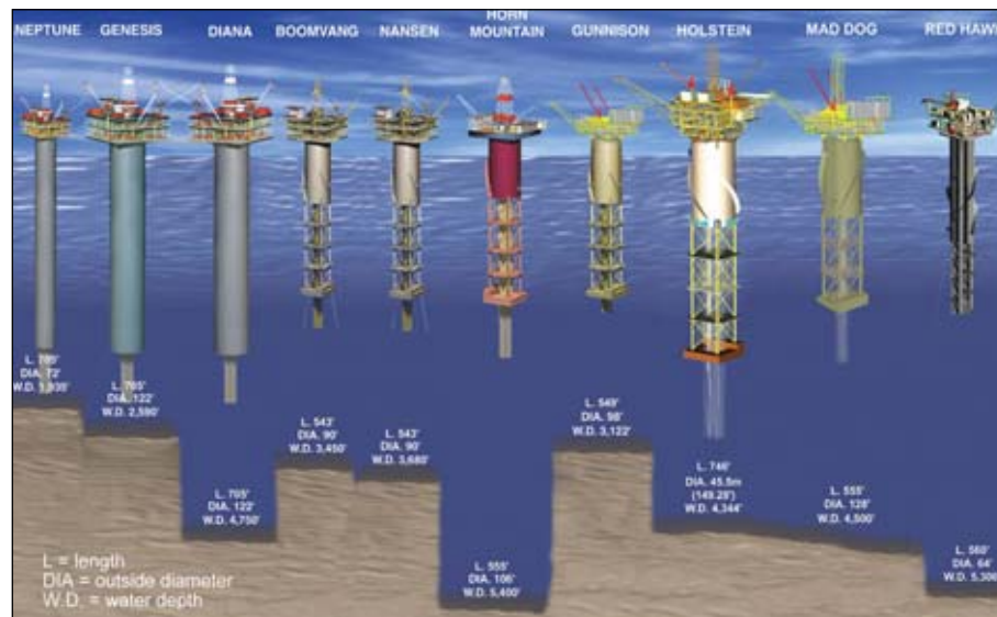
Progression of spar deepwater development systems.
