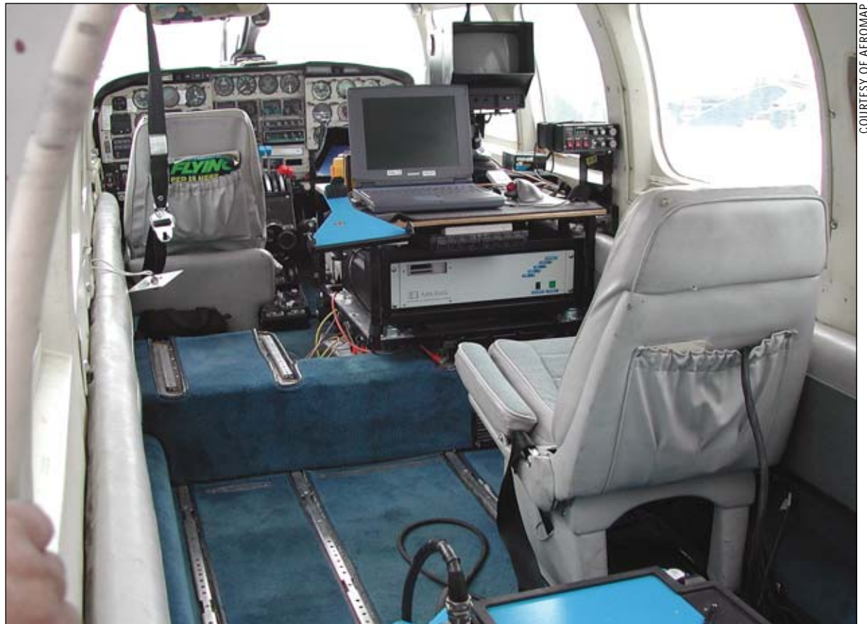
A Navajo Chieftain configured for airborne imaging surveys.
