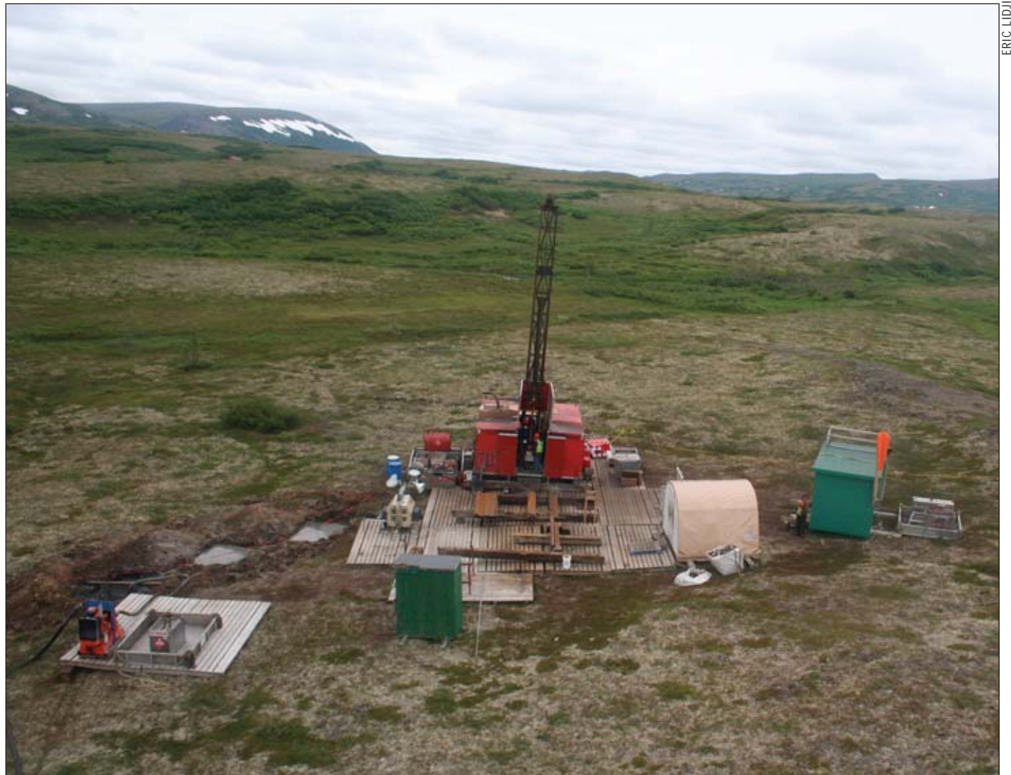
As engineers develop a mine plan for the Pebble project, drills will be moved into areas of potential development to collect geotechnical data needed to complete development plans.
