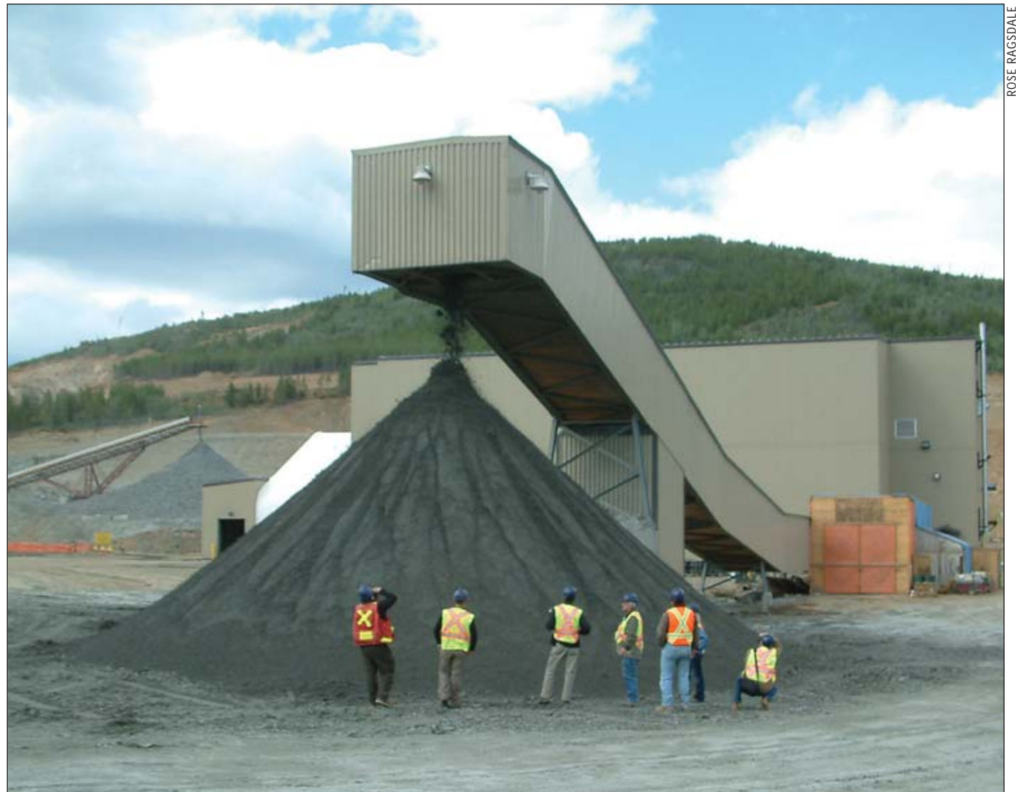
The ore processing system at the Minto Mine in central Yukon Territory dumps tailings containing significant amounts of copper and gold where mine owner, Capstone Mining Co., intends to return to extract more concentrates later after mining of high-grade deposits has been completed.
