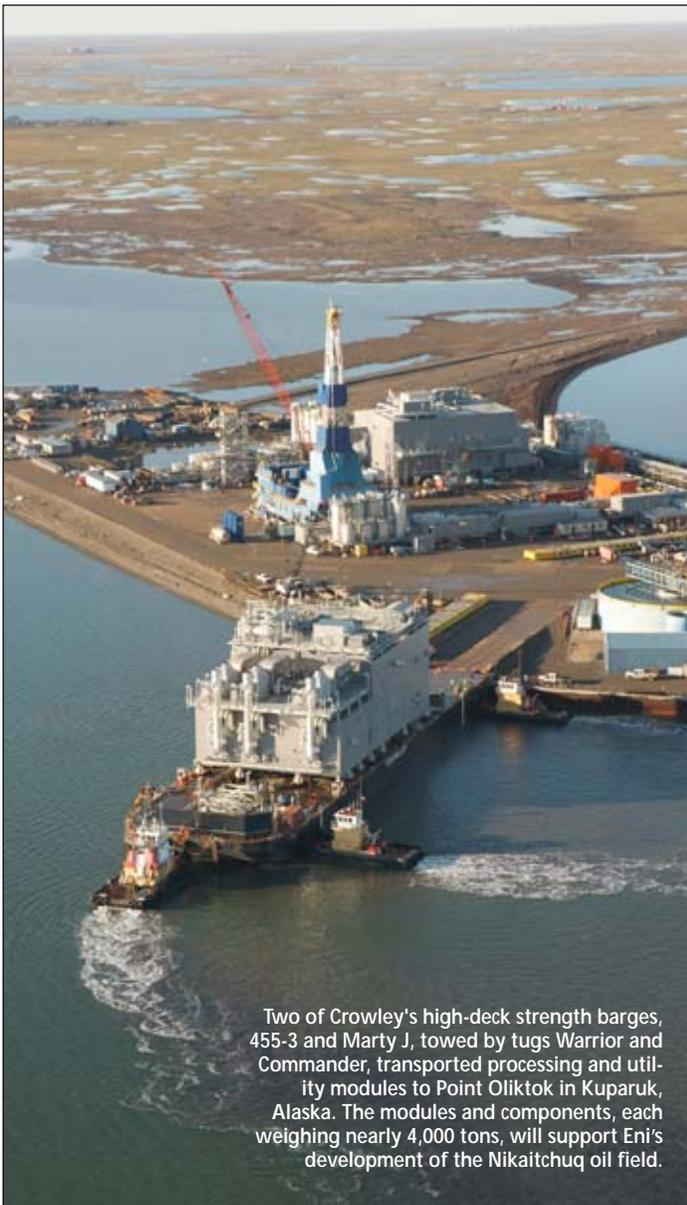
Two of Crowley's high-deck strength barges, 455-3 and Marty J, towed by tugs Warrior and Commander, transported processing and utility modules to Point Oliktok in Kuparuk, Alaska. The modules and components, each weighing nearly 4,000 tons, will support Eni's development of the Nikaitchuq oil field.
