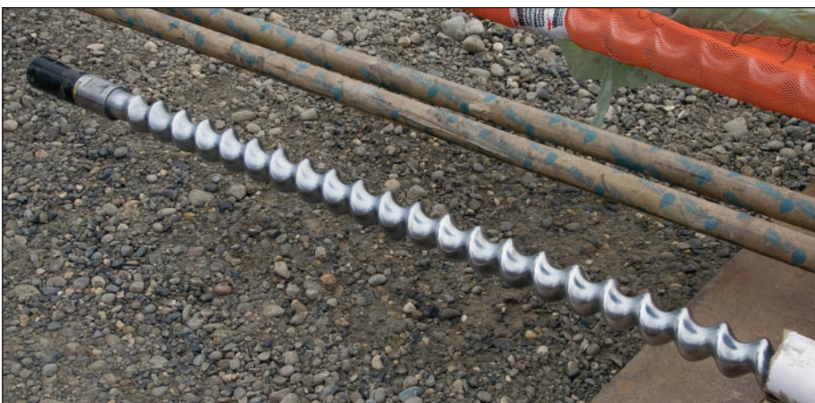
The auger-like rotor of the progressive cavity pump used to reduce the well downhole pressure and draw a mixture of sand and oil up the well.
