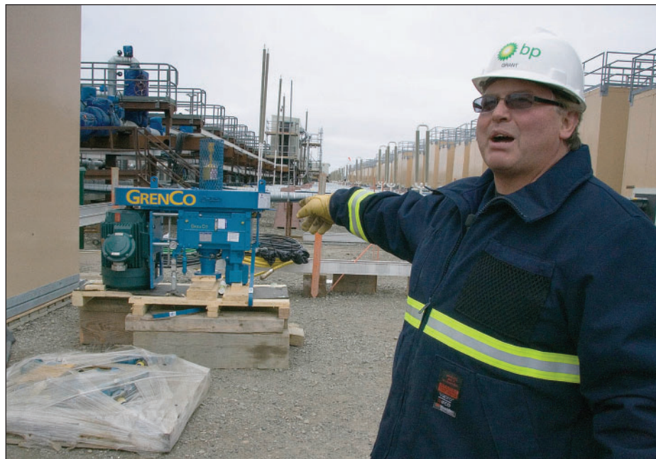
Grant Encelewski, operations lead tech for the BP heavy oil team, points to the top-drive motor unit for the downhole pump. The pump will be installed on the wellhead of the test well.
