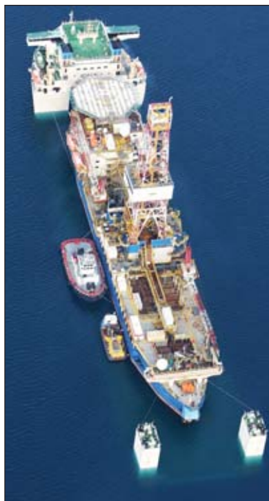
The heavy-lift vessel, the Xiang Yun Kou, submerges its cargo deck under the drilling vessel, Noble Discoverer, in Seward, prior to refloating with the drilling vessel on board.
