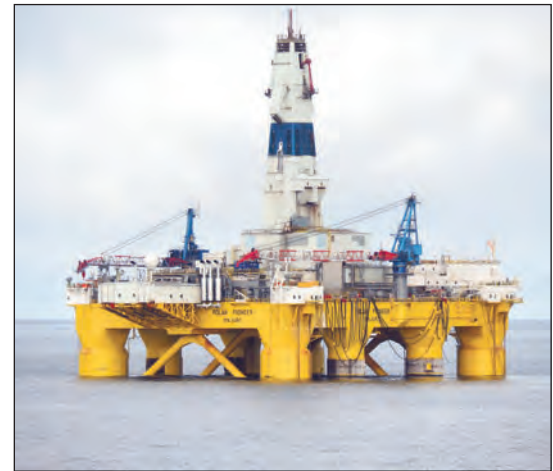
The semi-submersible drilling rig Transocean Polar Pioneer on location in the Chukchi Sea. The rig is drilling the Burger J well as part of Shell's Chukchi Sea exploration program.
