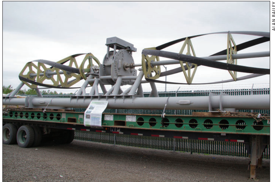
Ocean Renewable Power Co. has pioneered the use of helical in-water turbines for generating electrical power from water currents, in rivers or in regions with strong tidal currents.
