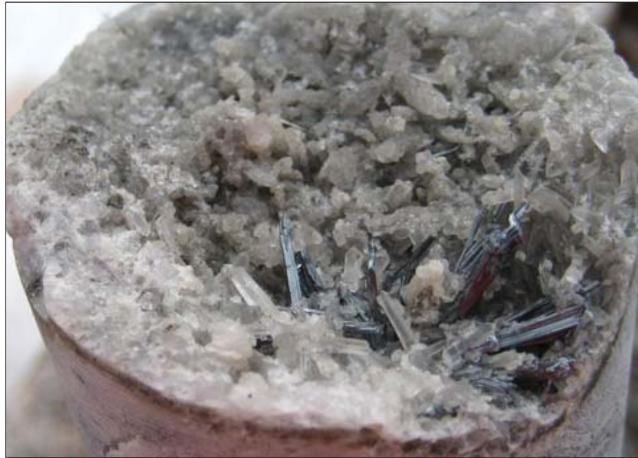
Crystals of stibnite (antimony sulphide - Sb 2 S 3 ) with quartz in drill core taken in 2007 from the Scheelite Dome Project in Yukon Territory.
