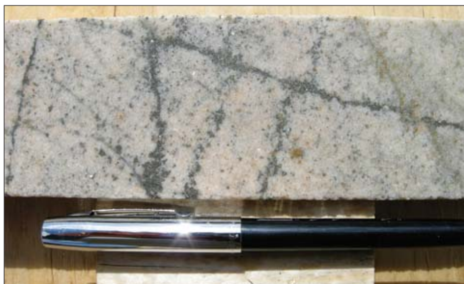
This sample, which contains quartz, albite, ankerite and sericite, plus fine disseminated and veinlet pyrite, averages 6.2 grams of gold per ton and is typical of the highly-altered mineralization found at Golden Saddle.
