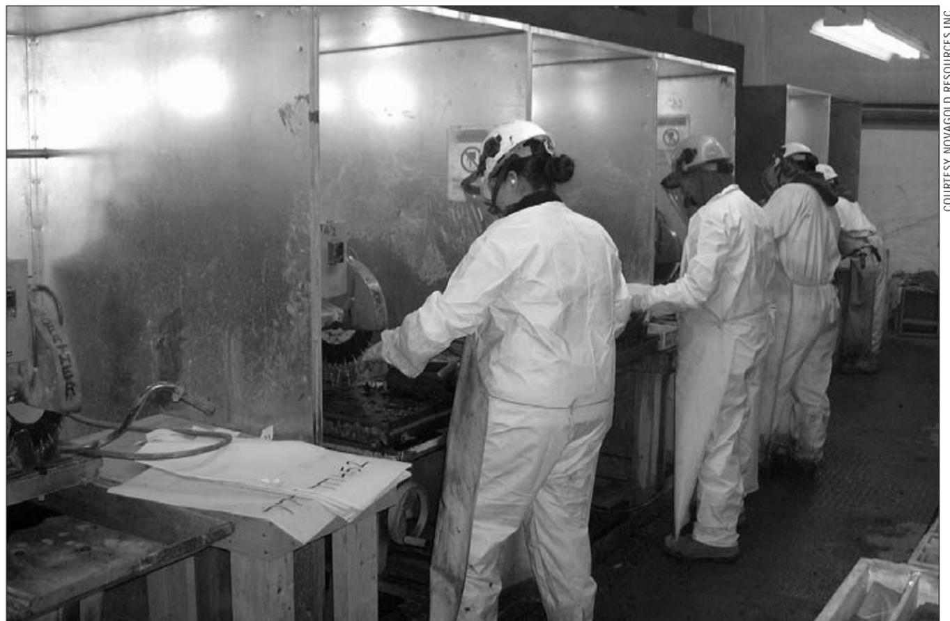
Workers saw drill core in an assembly line inside the core shack at the Donlin Creek gold project in 2007.
