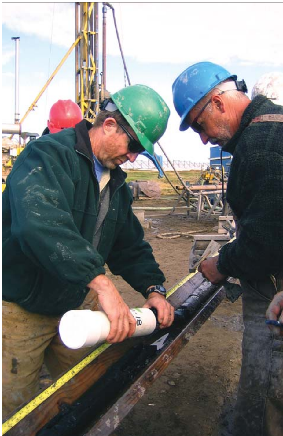
Placing a coal core from the Wainwright well into a PVC desorption canister.
