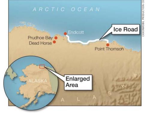
The sea-ice road to Point Thomson enabled the transportation of heavy equipment and materials for drilling operations while protecting the North Slope environment.
