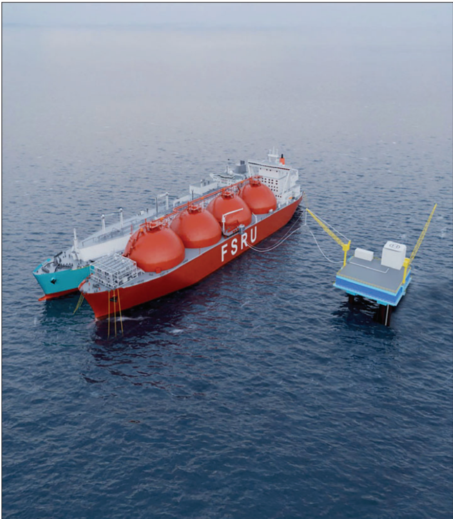
This rendering depicts a moored FSRU vessel connected to the Osprey platform in Cook Inlet. The Cook Inlet LNG project will utilize as much existing oil and gas infrastructure as possible to keep the development cost and timeline to a minimum.
