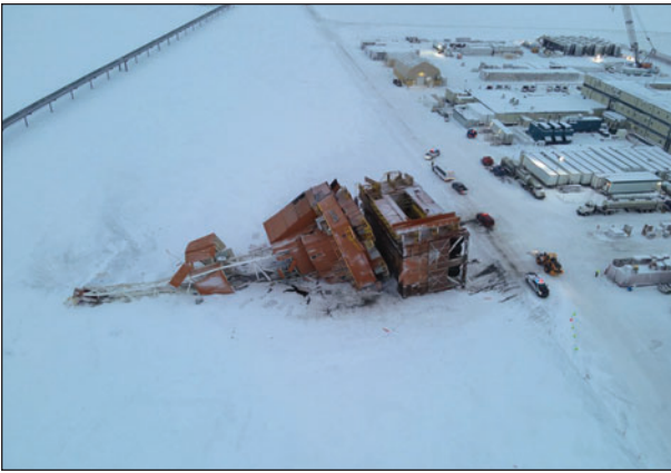
Rig 26, a self-propelled drilling module, left the road and toppled onto the tundra near “K pad,” which is a gravel pad owned by Kuukpik Corp. and leased by ConocoPhillips Alaska.
