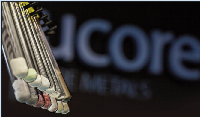
Rare earth element salts derived from a solution sourced from Ucore Rare Metals' Bokan Mountain project in Southeast Alaska.
