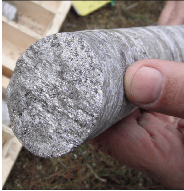
Core from drilling through the thick layers of high-grade graphite at the Graphite Creek project in western Alaska.
