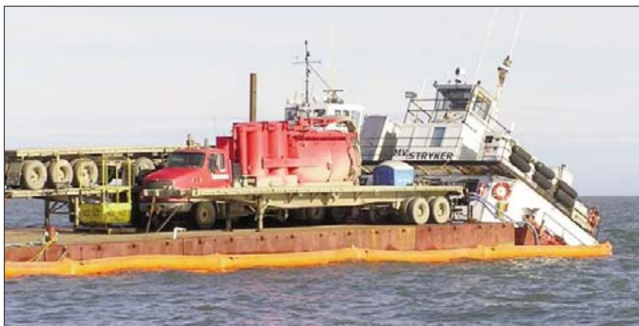
The vessel partially split, with the stern of the wheelhouse section drooping down and settling on bottom in 9 feet of water while the flatbed barge section at the bow remained afloat normally.
