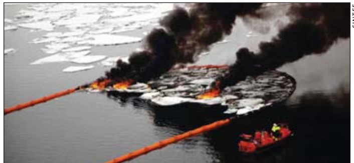
A controlled burn of oil in ice conditions in the Barents Sea, using fire boom to corral the ice and oil, demonstrated the effective removal of almost all of the oil.
