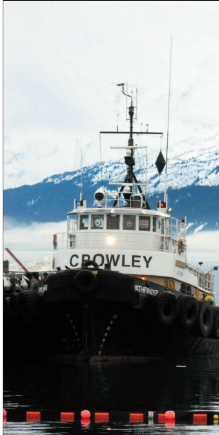
The tug Pathfinder, seen here anchored south of Busby Island in Prince William Sound after running aground Dec. 23 on infamous Bligh Reef. Boom encircles the vessel to contain diesel leaking from its ruptured fuel tanks.
