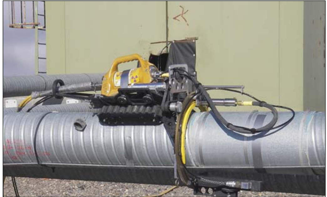
Envision ScanTrack is a robotic pipeline crawler inspecting pipelines for corrosion in real time.
