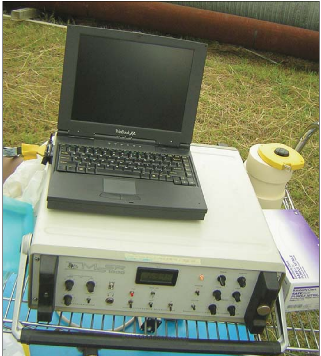
Guided Wave Ultrasonic system for longitudinal monitoring of cased piping.
