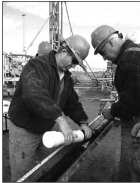
Placing a coal core from the Wainwright well into a PVC desorption canister
