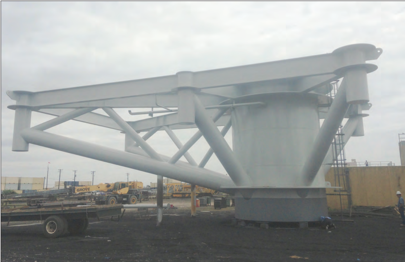
The platform support frame for Furie Operating Alaska's Kitchen Lights unit A platform.
