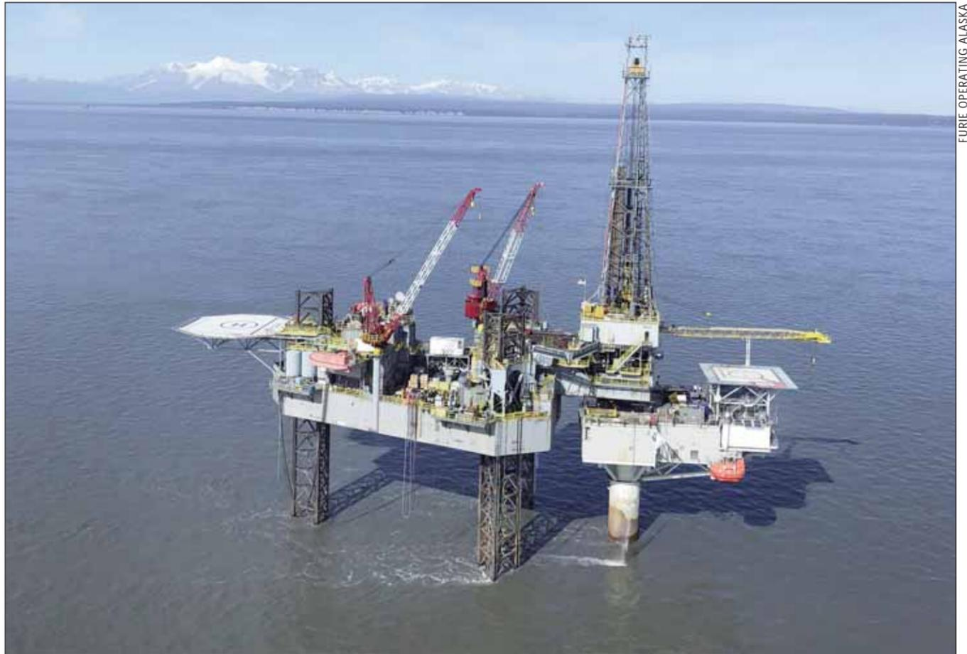
The Spartan 151 jack-up rig cantilevered over the Julius R. platform for development drilling in the Kitchen Lights gas field in the Cook Inlet.
