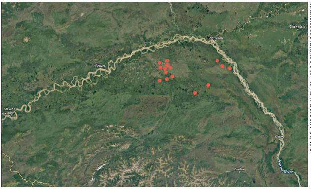
The locations of 15 potential Hilcorp stratigraphic test wells permitted by the Alaska Oil and Gas Conservation Commission for drilling in the Yukon Flats basin. The basin lies around the Yukon River, between the trans-Alaska pipeline and the Canadian border. The permitted well locations lie between the villages of Birch Creek and Fort Yukon, in the central part of the basin.
