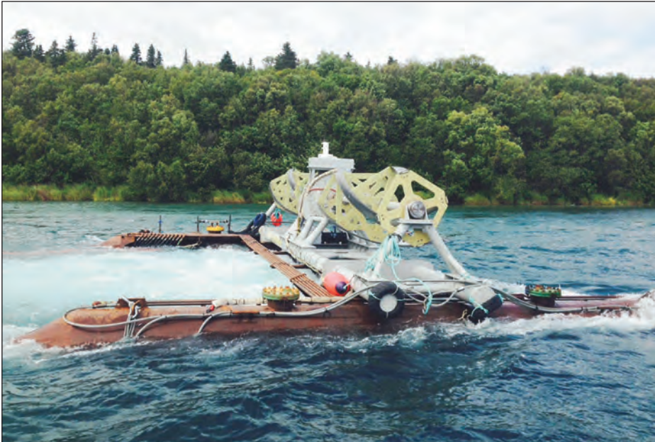
Ocean Renewable Power Co.'s RivGen being deployed in the Kvichak River during the summer. The device was sunk to the bottom of the river, enabling its helical shaped turbine to generate electricity for the village of Igiugig.
