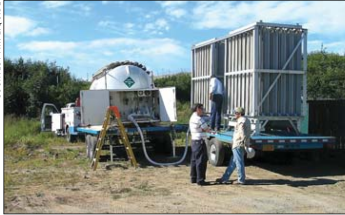
Mat Sanders, left, and Terry Rollings with Air Liquide's custom designed, small purge/pigging system.
