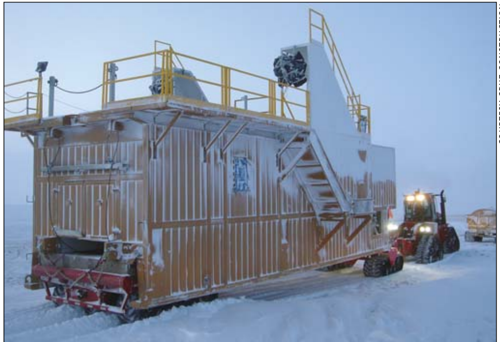
Cruz Construction recently completed the 270-mile move of the Doyon Arctic Wolf sub-base for FEX from Deadhorse west to its Amagaq location. FEX, part of Talisman Energy, began drilling in mid-February at the NPRA site. Steiger rubber track tractors were used to execute the move.
