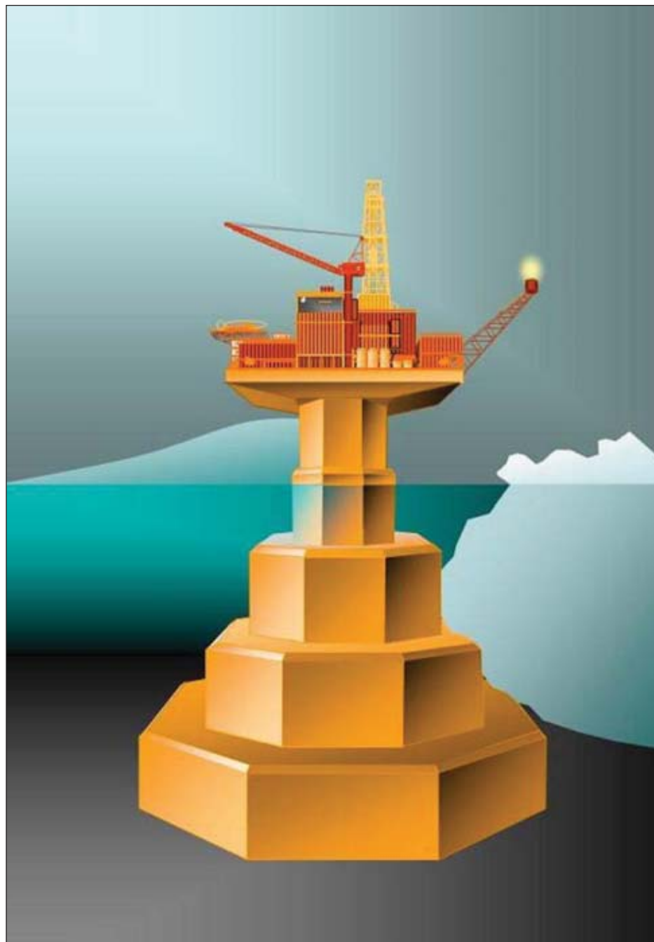
Massive steel structures that taper upwards are a possibility for oil and gas fields in the Beaufort and Chukchi seas.
