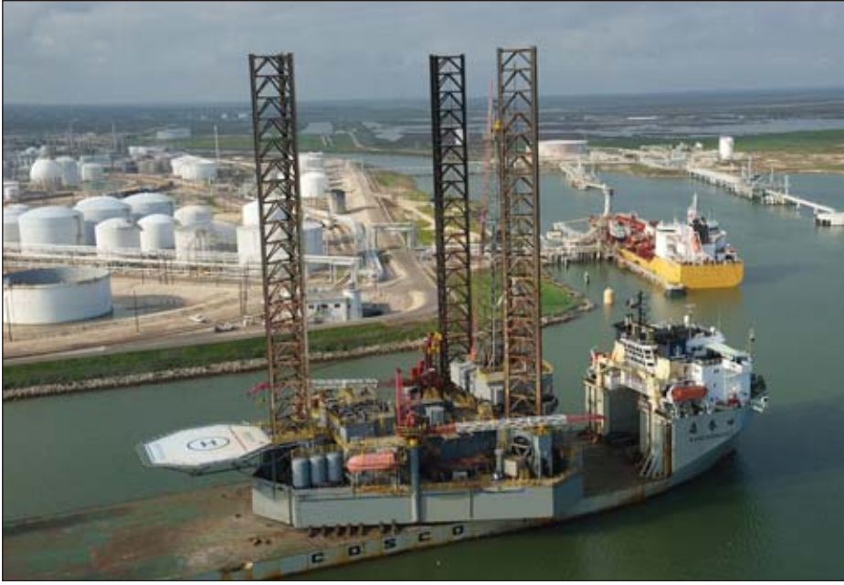
At the invitation of Escopeta President Danny Davis, the Spartan 151 jack-up underwent a preliminary inspection by State of Alaska officials prior to departure from Freeport, Texas. Final inspection will occur in Alaska after a 15,000-pound blowout preventer is installed on the rig.
