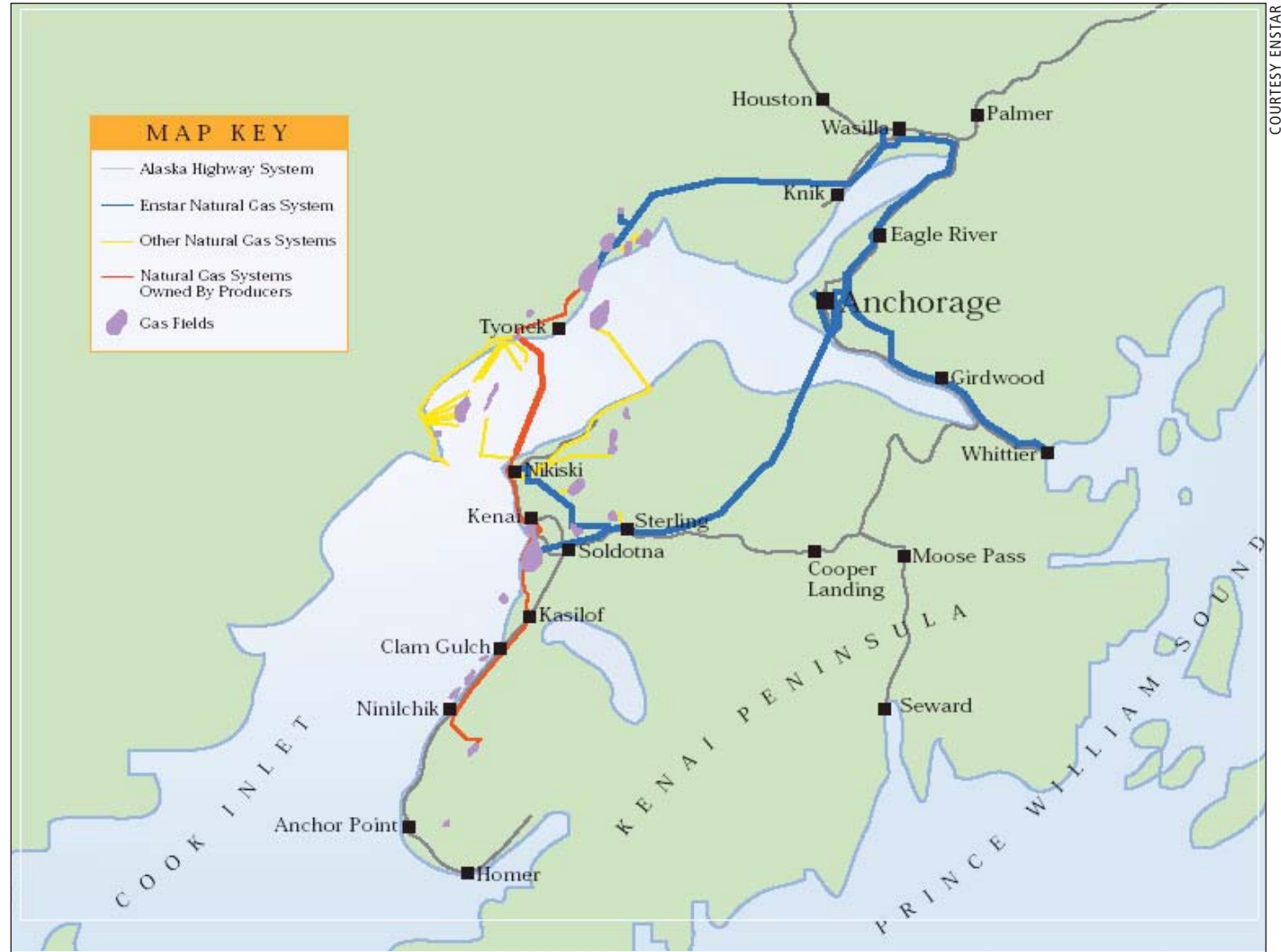
Gas pipelines in Southcentral Alaska (Enstar's pipeline are marked in blue). Potential extensions include a line from the North Slope into the northern end of the network, and a line south from Ninilchik to Homer.
