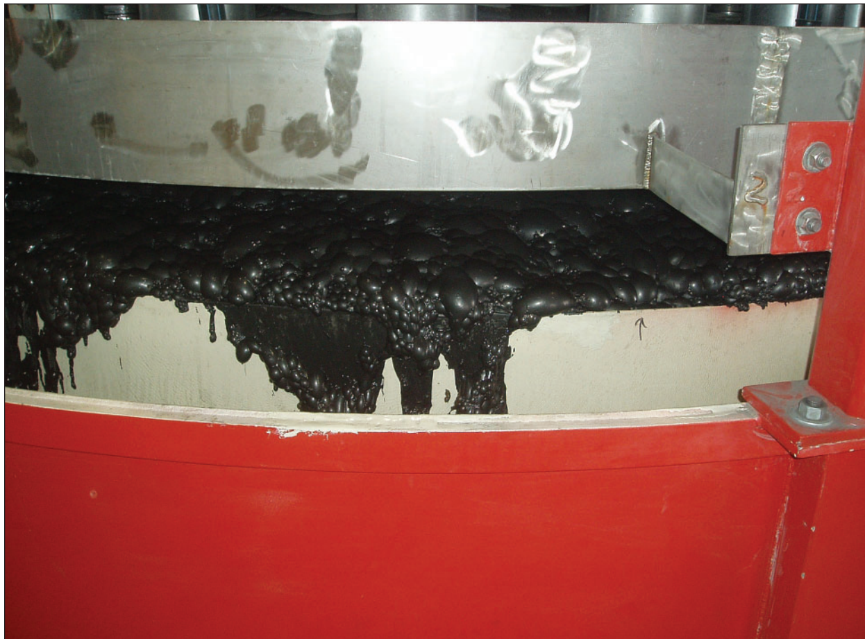
The new Jameson cell recycles material at a rate of 3,000-4,000 gallons per minute.
