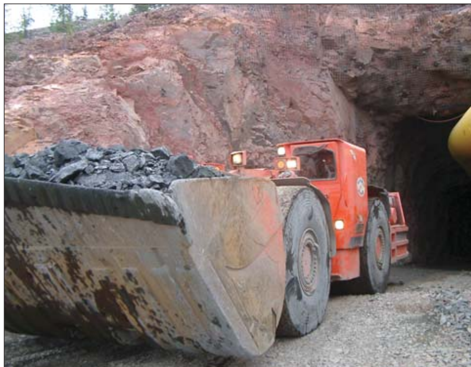
loaded scoop tram exiting the portal for the underground workings at the NICO project site.
