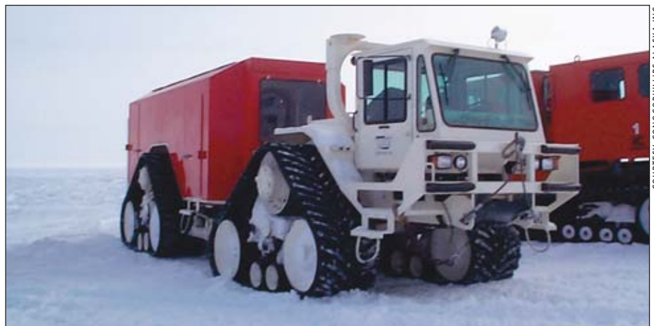
The evolution of vibroseis vibrator trucks between the 1980s and the early 2000s: Low-pressure rubber tracks with articulated steering have replaced steel tracks with skid steering.
