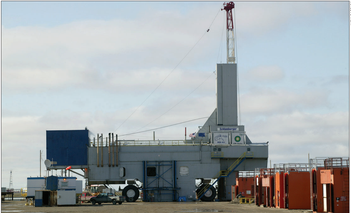
The cantilevered drilling platform on a rig such as the Nordic-Calista No. 2 rig, shown here, minimizes the spacing necessary between the wellheads on a well pad.
