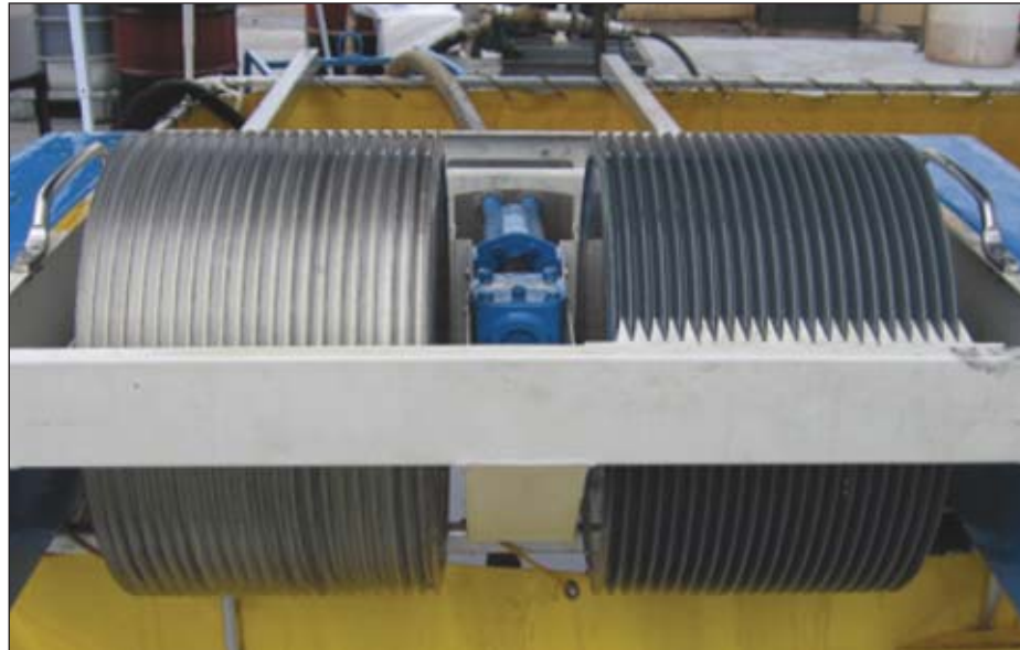
Drums used to test new drum coating materials in University of California Santa Barbara research.
