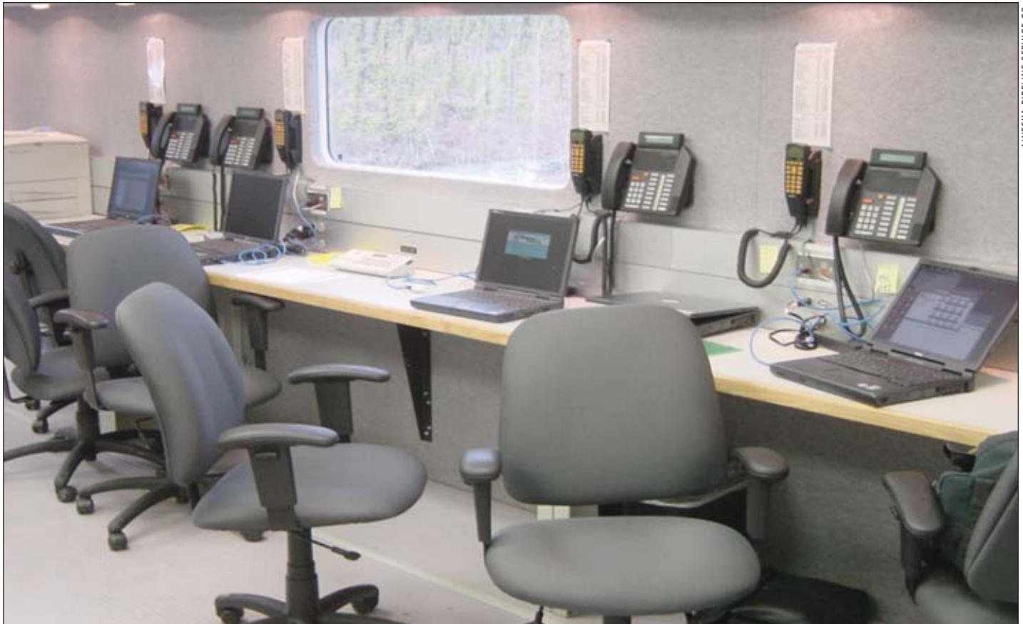
The MCP has eight workstations with computers, laptops, satellite phones, regular telephones and a dispatch center with air and ground radios as well as different repeaters.
