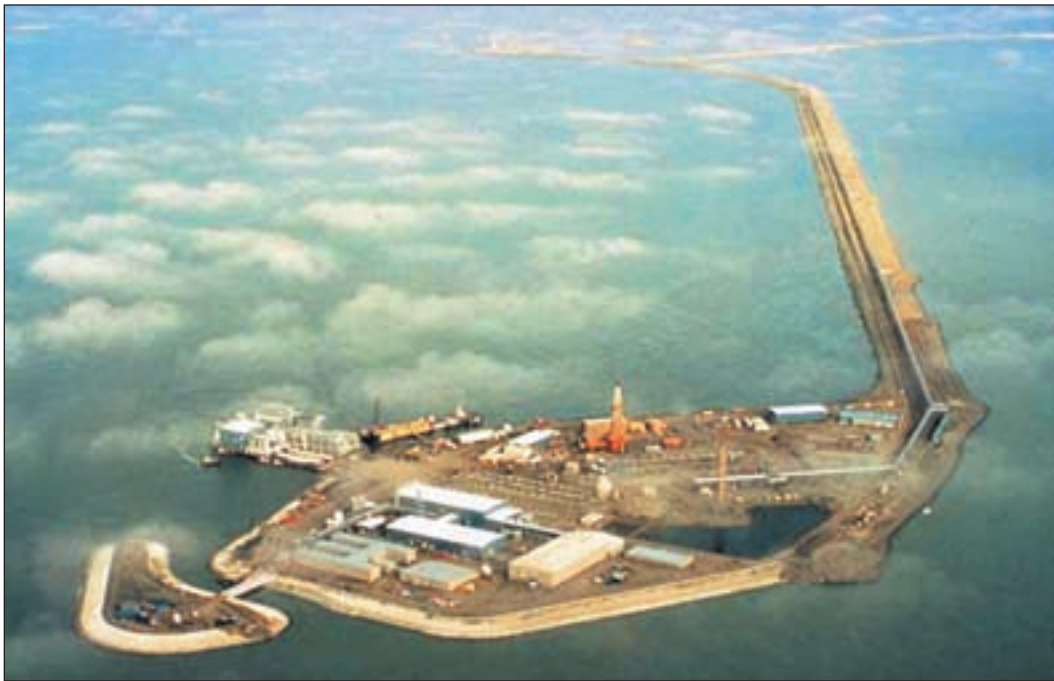
Alaska holds the honor of producing the first oil from Arctic waters: BP's Endicott oil field in the Beaufort Sea. Northeast of Prudhoe Bay, Endicott is connected to the mainland by a 1.5-mile gravel causeway.
