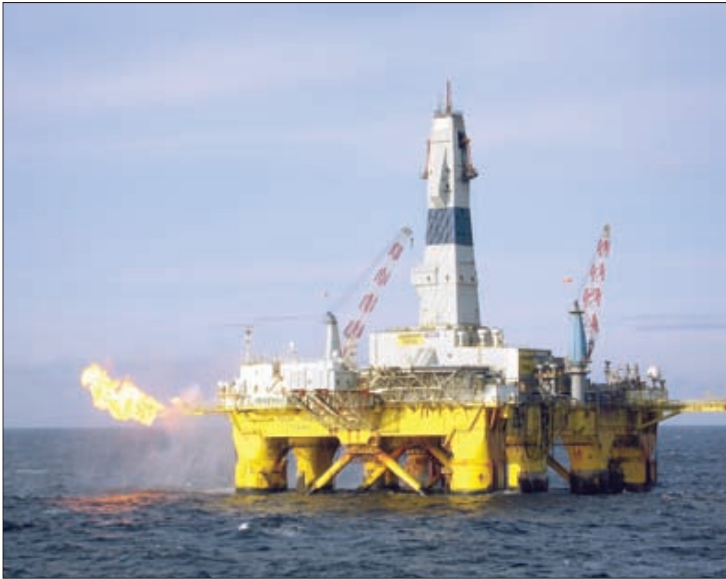
The first Snohvit well was completed by Transocean's Polar Pioneer semi-submersible rig, which Statoil said would perform the same operations on the remaining eight production wells and a carbon dioxide injection well drilled through Snohvit's four seabed templates.
