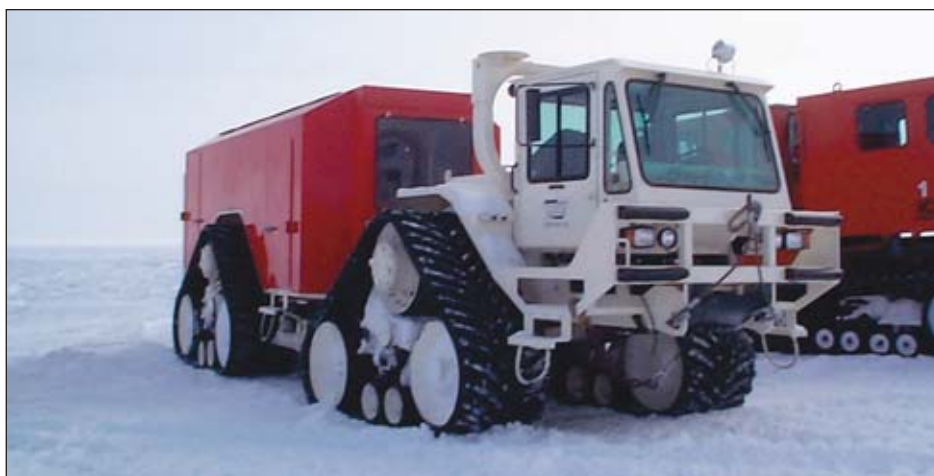
The evolution of vibroseis vibrator trucks between the 1980s and the early 2000s: Low-pressure rubber tracks with articulated steering have replaced steel tracks with skid steering.
