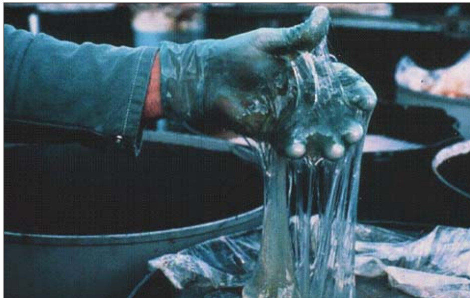
A worker dips a hand into a batch of drag reducing agent, or DRA. The chemical additive has proven to be an important boon to operators of the trans-Alaska oil pipeline.
