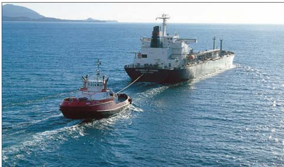
The Nanuq, one of two enhanced tractor tugs operated by Alyeska Pipeline Service Co., is tethered to the stern of the oil tanker American Progress as it heads for the open ocean beyond Prince William Sound. Alyeska's new emergency prevention priority requires tug operator Crowley Marine Alaska to keep a line attached to oil tankers under way through the Sound.
