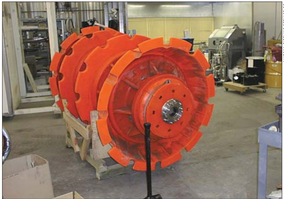
This paraffin cup scraper pig is used to clean wax buildup from the walls inside the trans-Alaska oil pipeline. It is one of three types of cleaning pigs used on the trans-Alaska oil pipeline and the one Alyeska Pipeline Service Co. uses most often.
