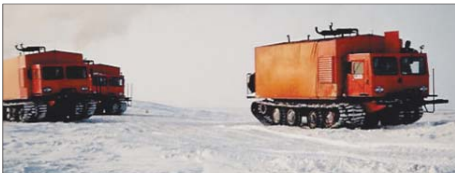
The evolution of vibroseis vibrator trucks between the 1980s and the early 2000s: Low-pressure rubber tracks with articulated steering have replaced steel tracks with skid steering.
