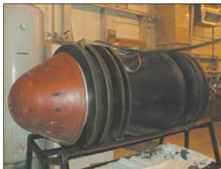
This pig has hard plastic discs for aggressive cleaning. Alyeska Pipeline Service Co. technicians run them through sections of the 800-mile trans-Alaska oil pipeline as needed.
