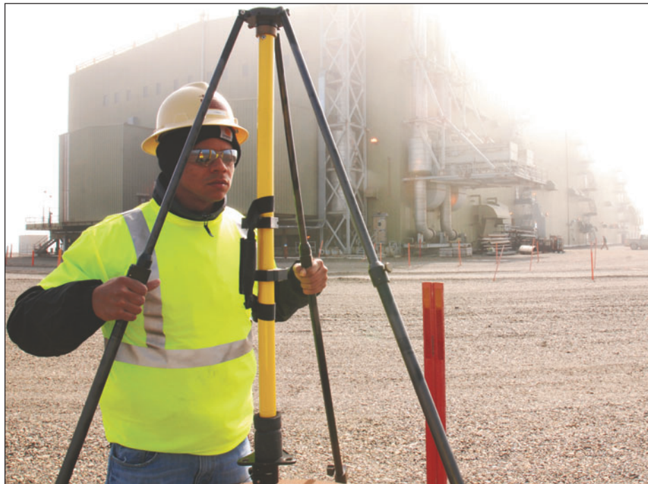
Fugro survey team sets control for a shallow hazards program on the North Slope.
