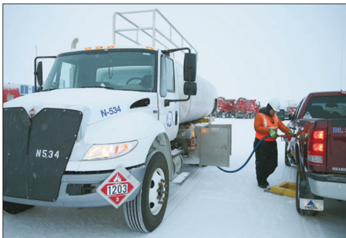
All fueling is done on-site for vehicles and machinery, and is hauled approximately 65 miles from Deadhorse to the storage tanks at the Qugruk Camp pad. Extra care is taken that no fuel drips onto the ice pad.
