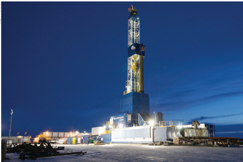
Mobile, lightweight drilling rigs, such as Nabors 105E (pictured), have reduced North Slope exploration costs.
