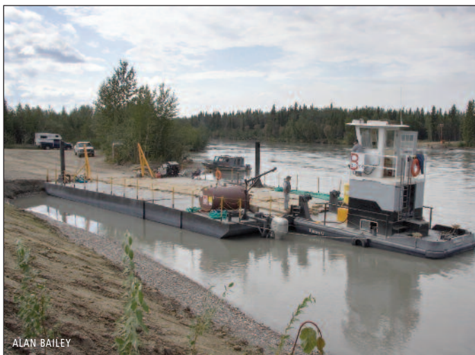
A group of companies drilled a well in the Nenana basin in 2009. A barge stationed on the Nenana River was used to carry heavy equipment across the river to the drillsite access road, seen directly behind the barge.
