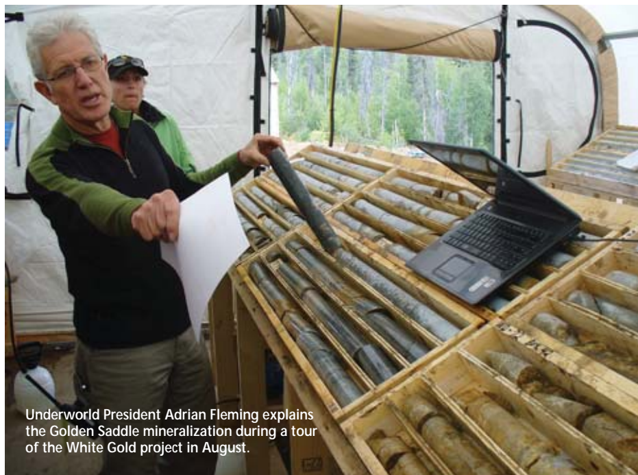
A core segment from hole WD09-44, drilled into the Golden Saddle zone, encountered 56.1 meters averaging 3.91 g/t gold, including 32.5 meters averaging 5.58 g/t gold.
